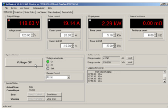
Manual control window with charge/energy counter
